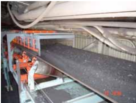
Martin® ApronSeal™ Skirting was installed on the outside of the new 12-inch (304-mm) skirtboard.
