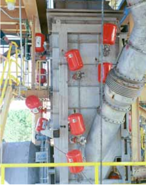
Martin® Air Cannons were installed on the pre-heater to maintain material flow into the kiln.
