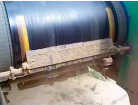
The Martin® SHD Cleaner is built to stand up to fast belts and heavy material loads.
