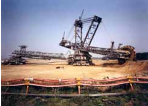
Bucketwheel excavators and high-capacity conveyors are used in Rheinbraun's lignite mining operations.
