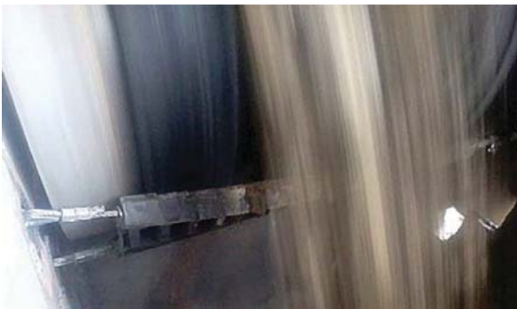
The blade spans the entire length of the belt, cleaning from edge to edge for more efficient operation.
