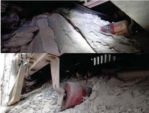
Excessive carryback adhered to the return side of the belt and encapsulated idlers.
