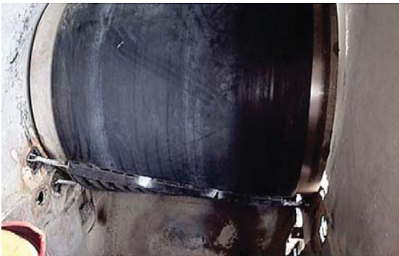
With its small footprint, the CleanScrape® Cleaner is set diagonally on the head pulley.
