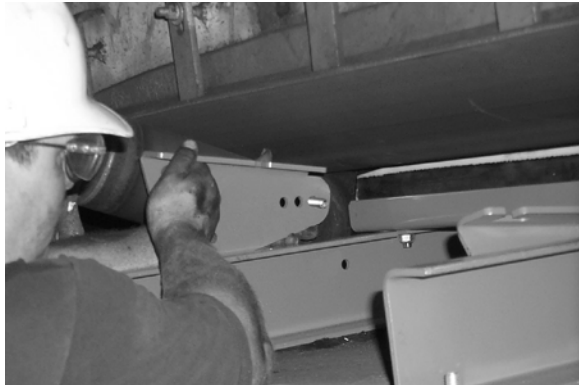
14. Bolt wings in the correct holes but do not tighten.
