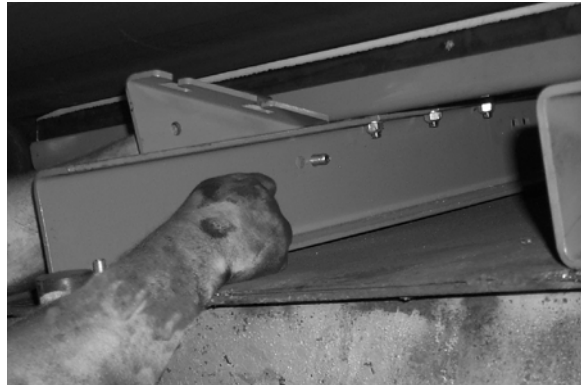
14. Bolt wings in the correct holes but do not tighten.
