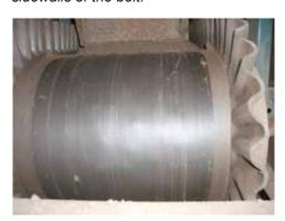
Following installation of the Martin® QC1™ Cleaner HD, the corrugated sidewall belts on the weigh feeders were much cleaner.
