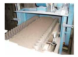
The plant's weigh feeders suffered carryback as a result of an inability to effectively clean the sidewall belts.
