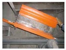
The Martin® QC1™ Cleaner HD was installed on a modified mainframe to provide effective cleaning without interference from the sidewalls of the belt.
