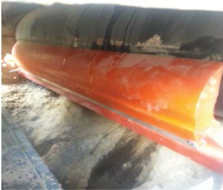
The Patented "CARP" Constant Angle Radial Pressure design keeps a tight seal on the belt.
