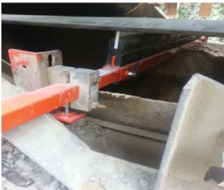
Martin® SC16 Cleaner uses a tungsten blade to dislodge adhered material.
