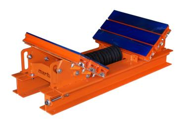
Installed under a belt conveyor loading zone, the <u>Martin</u>® <u>Combination Cradles</u> absorb the force of falling material to prevent damage to the belt and structure. The impact cradles stabilize the belt line to prevent material escape.
