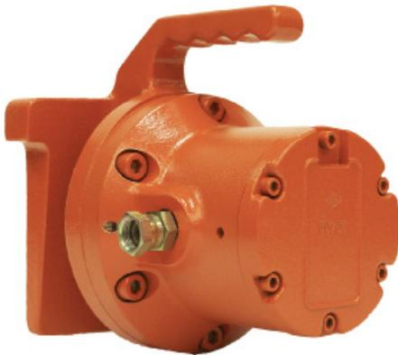
The **Martin® Impacting Railcar Vibrator** delivers a powerful force output of 3400 lbs at 80 psi while only weighing 48 lbs, making it the highest-force, lowest-weight portable railcar vibrator available. The Martin® Impacting Railcar Vibrator provides the force required to activate the free flow of tough materials that are sticky, coarse, and high in moisture.
