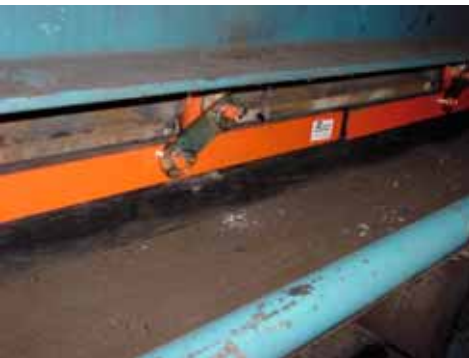
Available with rubber strips up to 300 feet (91 m) long, Martin® Self Adjusting Skirting provides a continuous joint-free seal.
