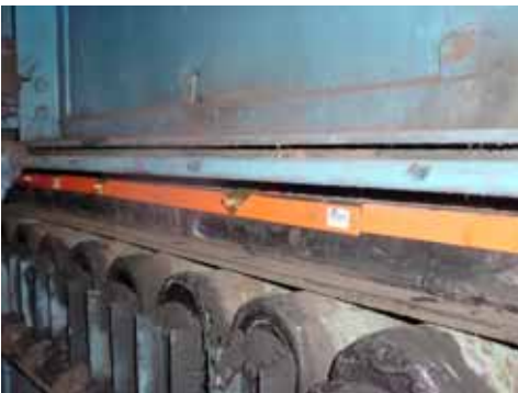
Martin® Self Adjusting Skirting works on conveyors with as little as 1.25 inches (32 mm) of free belt space outside the steel chute.
