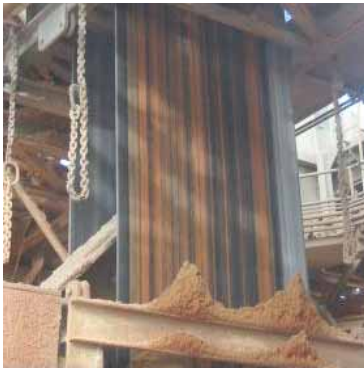
The parallel conveyors at the La Quinoa Agglomeration Plant provided the opportunity for comparative testing of belt cleaner performance.
