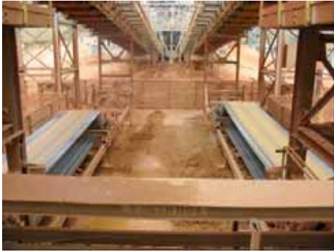
The parallel conveyors at the La Quinoa Agglomeration Plant provided the opportunity for comparative testing of belt cleaner performance.
