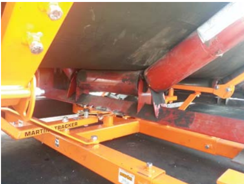
The Martin® Tracker™ Reversing helps cure wandering belts - in both directions.
