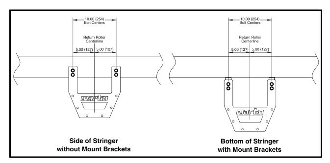
Figure 1. Martin<sup>®</sup> Return Roller Basket Mounting Location
