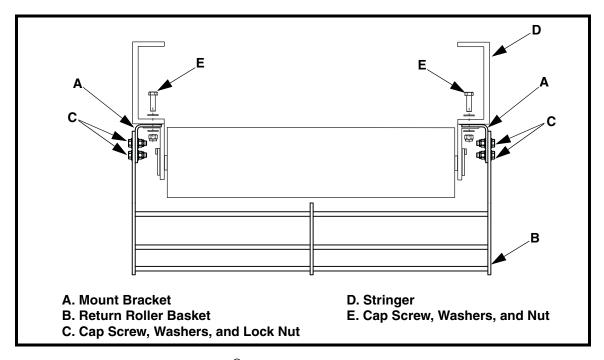
Figure 3. Martin<sup>®</sup> Return Roller Basket with Brackets
