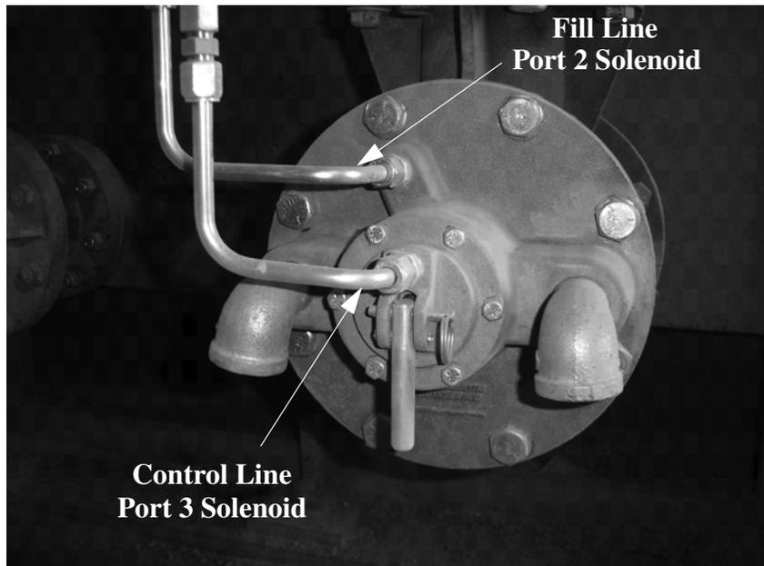
10. The original normally-opened solenoid line will be used as the new air fill line.
