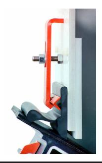
Martin<sup>®</sup> ApronSeal™ Single Skirting is a dual sealing system that prevents spillage without requiring service to maintain an effective seal. Martin<sup>®</sup> ApronSeal™ Skirting Systems provide dual-sealing surfaces. The primary seal is clamped to the chute wall with the self-adjusting secondary laying outward to create an effective dust seal that is out of the material flow.
