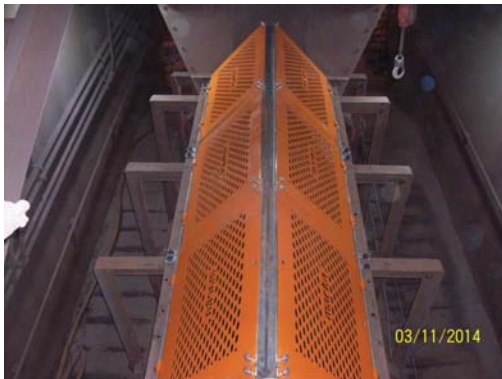
Martin® Conveyor Guards prevent material from spilling off the belt.
