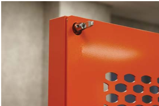
Wedge clamps allow the conveyor guards to be removed and reinstalled quickly without the use of tools.
