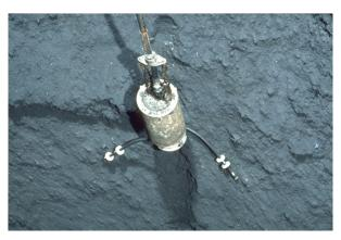
The Martin® Heavy Duty Whip is used to safely and quickly remove hardened, non-flowing material from silo walls and feeders.
