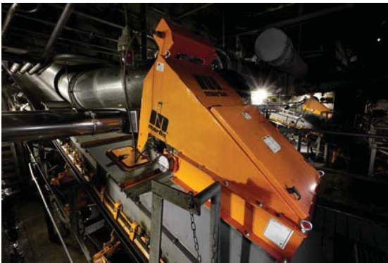
The Air Cleaner is installed above the transfer to capture airborne dust, collecting particles and returning to cargo.
