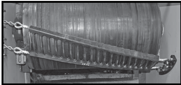
Correct Mounting Position
