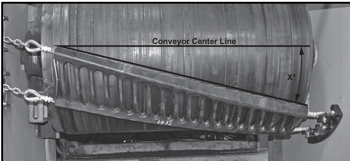
Figure 7. Measure Cleaner Angle
