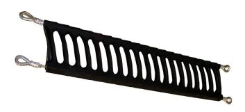
The Martin® CleanScrape is mounted diagonally on the discharge pulley and forms a three-dimensional curve. The cleaner has a matrix of tungsten carbide scrapers incorporated into the main rubber body during the vulcanization process. Despite a relatively low contact pressure between the belt and cleaner 85 to 95% of the adhering material is removed.
