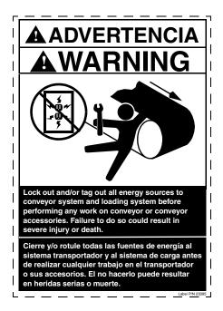
Figure 3. Conveyor Products Warning Label, P/N 23395
