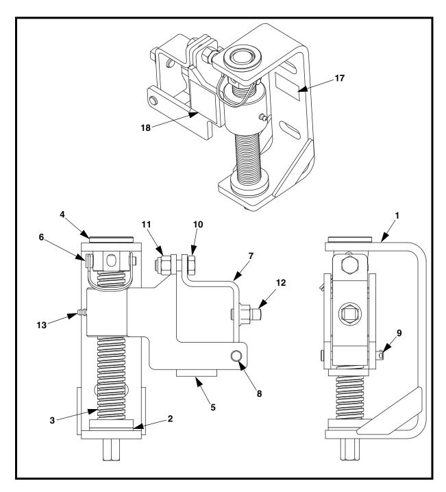
Figure 2.  $Martin^{\text{(B)}}$  SQC2S<sup>TM</sup> Square Mainframe Tensioner HD Assembly, P/N 38664-HD
