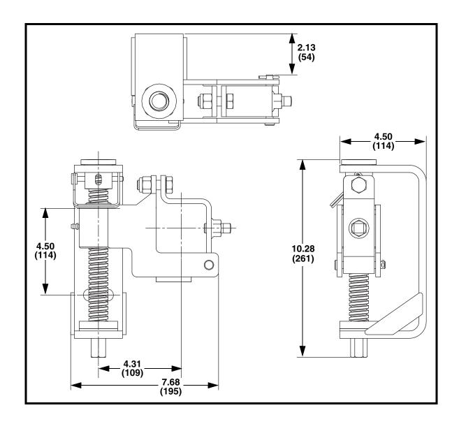
$Martin^{\text{(B)}} \ SQC2S^{\text{TM}} \ Square \ Mainframe \ Tensioner \ HD \ Assembly \ Dimensions$
