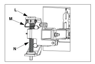
2. Align holes on threaded rod (N) with holes in top bushing (L) and insert pin (M).
