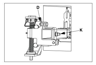
7. Tighten nut (D) and set screw (K).
