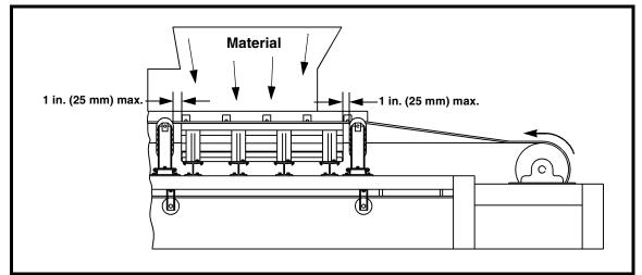
Figure 3. Installing Idlers with Martin® Impact Cradle or Support Cradle
