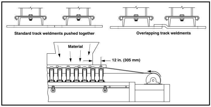
Figure 2. Installing Idlers in Impact Zone
