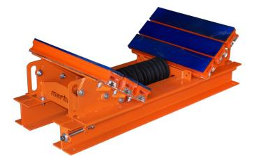
Installed under a belt conveyor loading zone, the <u>**EVO® Combination Cradles**</u> absorb the force of falling material to prevent damage to the belt and structure. The impact cradles stabilize the belt line to prevent material escape.
