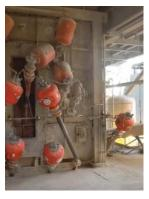
After - Martin installed blow pipes up through the ceiling to the floor above, making access easier.
