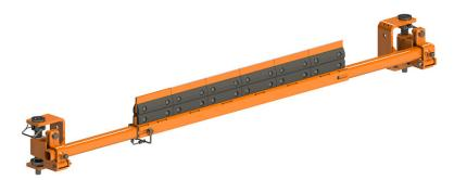
The Martin® SQC2S™ Reduced Mini Cleaner incorporates individually-cushioned tungsten carbide blades for effective cleaning without risk to belt, splice, or blade. Installed in the secondary cleaner position, the Martin® SQC2S™ Cleaner's blade buffers cushion impact and maintains cleaning pressure.
